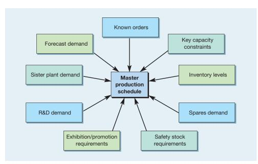
Figure 14.5 Inputs into the master production schedule
