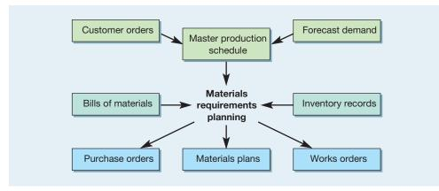
Figure 14.4 Materials requirements planning (MRP) schematic
