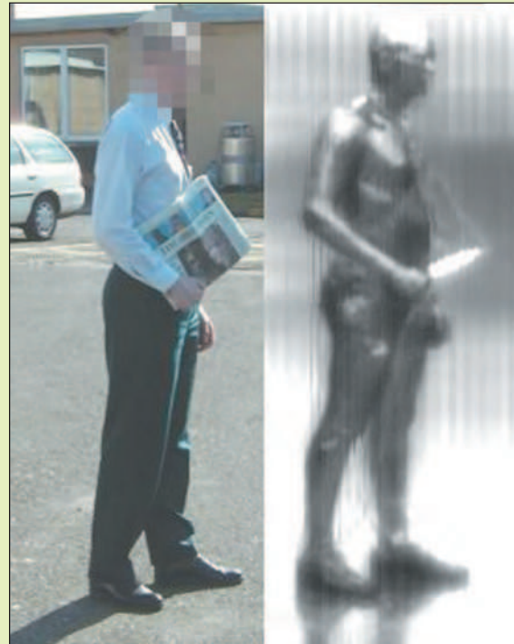
QinetiQ's 'Millimetre Wave' technology reveals that this man is carrying a knife
